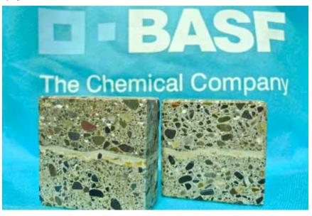
The MASTERSEAL<sup>®</sup> 345 waterproofing membrane is capable of bonding to both sides of the concrete substrates. pants.
