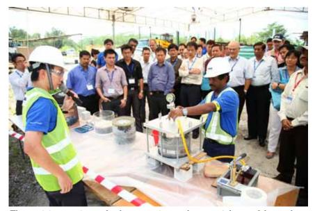
The participants witness the demonstration on the watertighness of the sandwich panel waterproofed with MASTERSEAL<sup>®</sup> 345 under a hydrostatic pressure of up to 4 bars.
