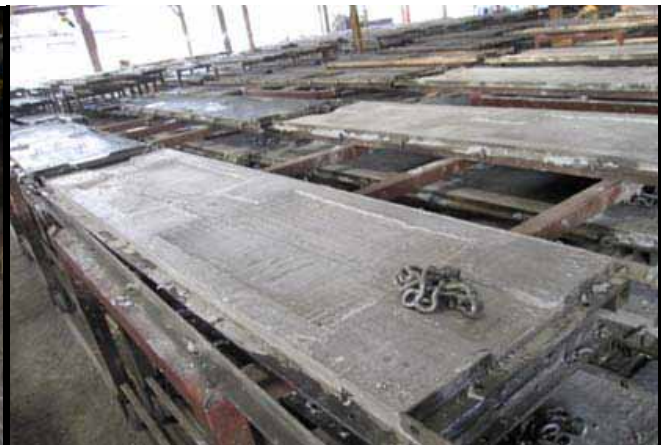
Adjustment of wall thickness by varying the torque applied to the connecting bolts
