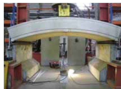
Figure 8. Segment Tests under Flexure in NTU.
