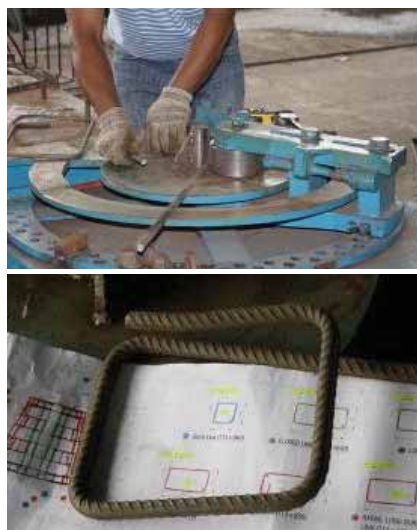
Figure 2. Worker using bar-bending machine to form links.
