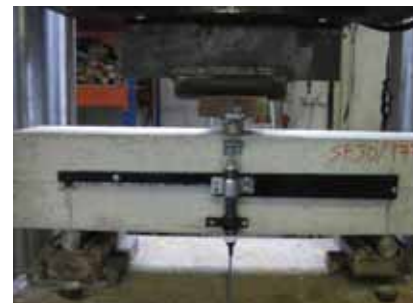
Figure 7. SFRC Flexural Tensile Tests in NTU.
