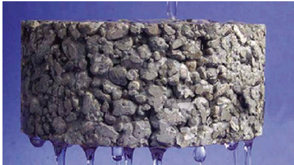
Fig. 2 : A core from pervious concrete
