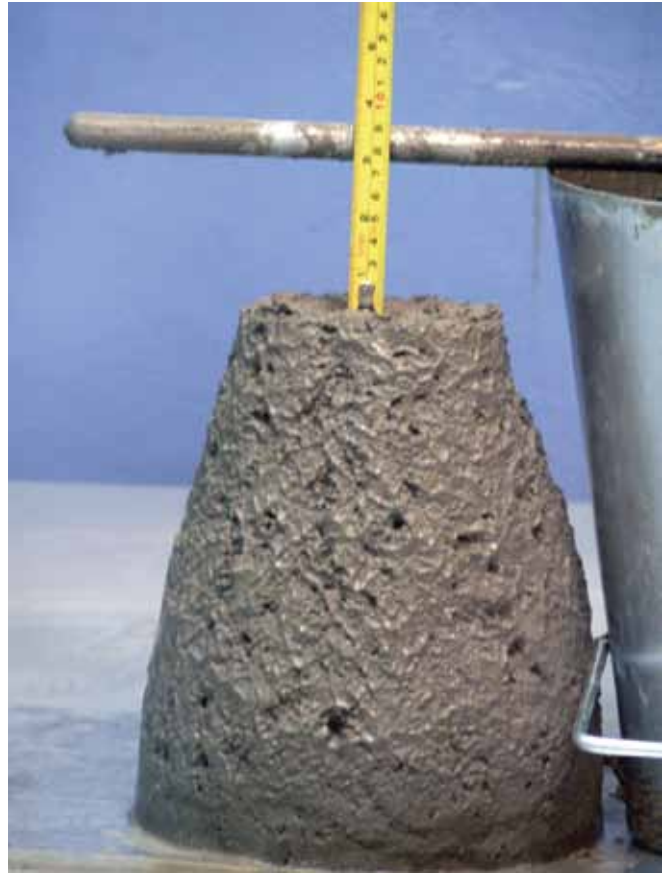
(L) Conventional concrete and (R) Concrete with super retention technology at 90 min elapsed time
