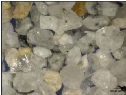
Figure 6: Particle Shape of VSI M-sand (Microscopic picture of Particle size: 1.18 mm to 0.60 mm)
