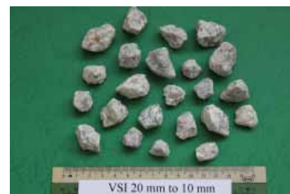
Figure 4: Picture of Particle Shape of VSI 20 mm Aggregate
