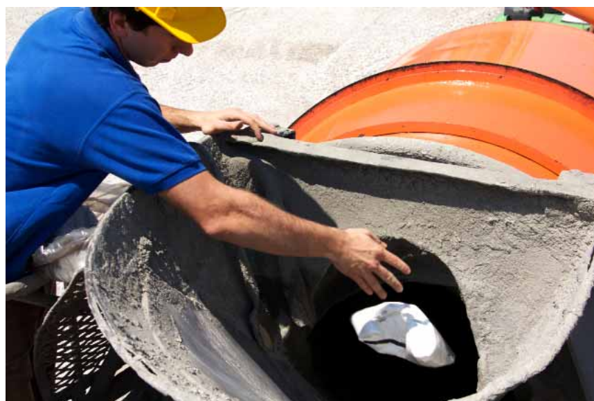
Figure 4 – A RE-CON ZERO kit to treat 1 m 3 of returned concrete comprises 7 water soluble bags (one 0.5 kg bag of Part A and six 1 kg bags of Part B).
