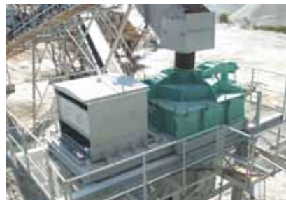
Figure 9: External View of Vertical Shaft Impact Crusher System (VSI)
