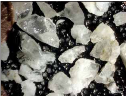
Figure 7: Particle Shape of Non-VSI M-sand (Microscopic picture of Particle size: 1.18 mm to 0.60 mm)
